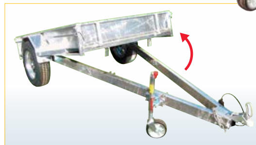
CT8x4TD and 8x5TD – single axle, tipping option
