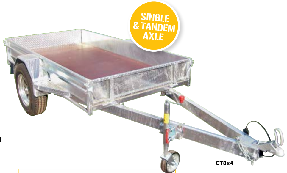
Front and rear tailgates become ramps
